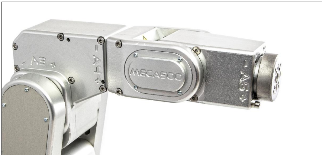
The Meca500 has six degrees of freedom and weighs only five kilograms. The controller is integrated into the base. Images ©Mecademic
