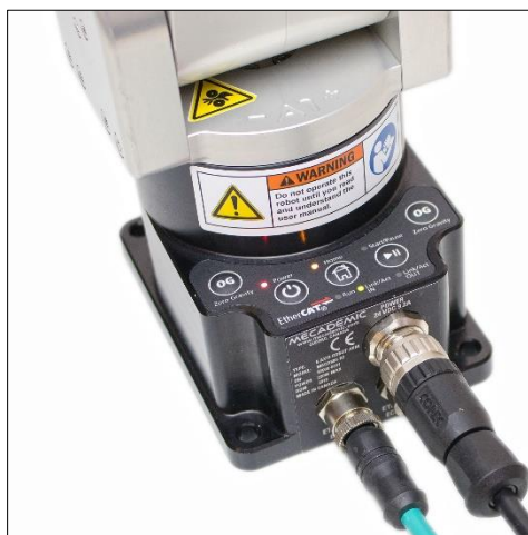
The Meca500 has six degrees of freedom and weighs only five kilograms. The controller is integrated into the base. Images ©Mecademic
