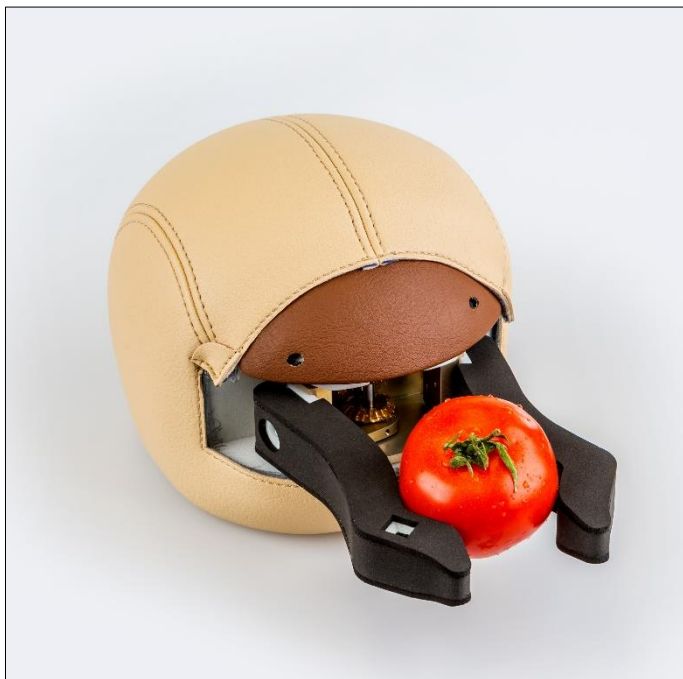
The robot's head can be fitted with various manipulators. Image © maxon motor
