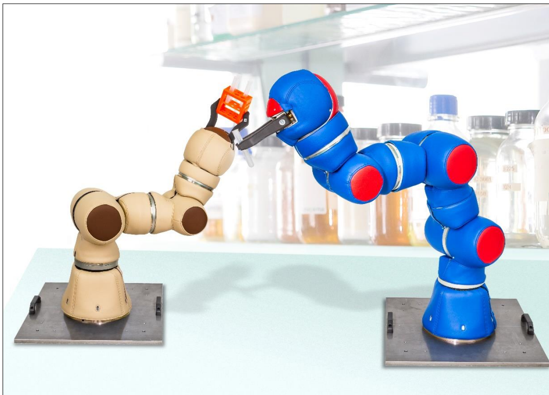
P-Rob 1R with six degrees of freedom (right) and 1U, a smaller-sized version. Image © maxon motor
