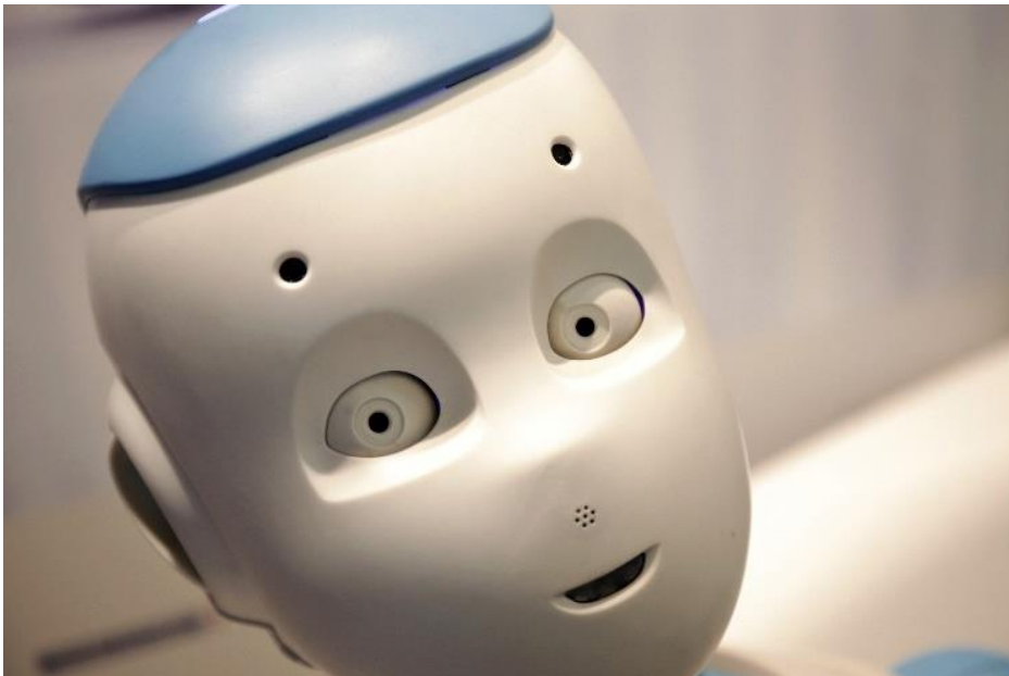
Romeo is an assistive robot, designed for helping elderly persons in their households (see image on page 1). DCX motors move his eyes. Images © 2014 Aldebaran
