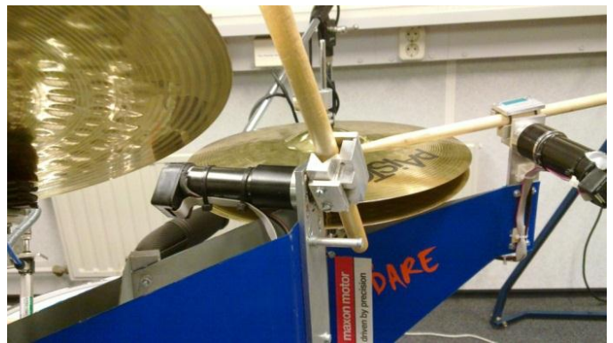
Figure 3: The crash and hi-hat of the drum kit are equipped with one maxon drive each. © 2011 TeamDARE
