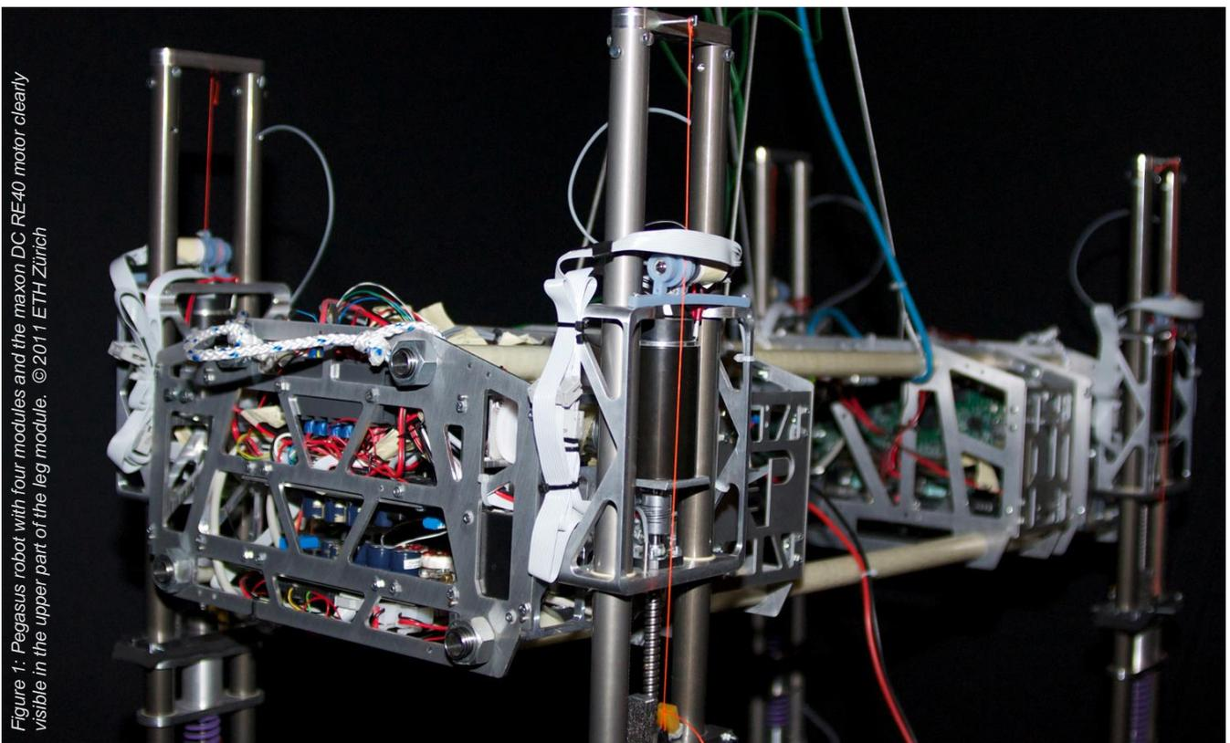
Figure 1: Pegasus robot with four modules and the maxon DC RE40 motor clearly visible in the upper part of the leg module. © 2011 ETH Zürich
