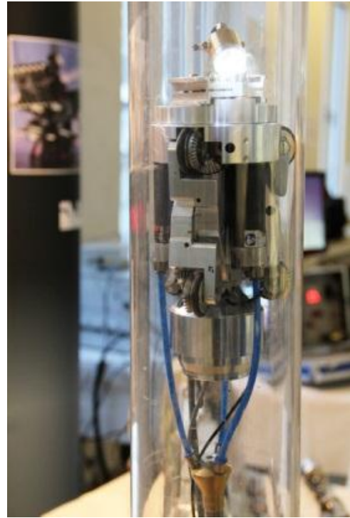
Figure 2: Plexiglas pipes provide a good view of the movement and functional principle of the manipulators. © 2012 Ibass
