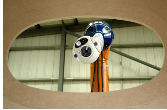
Figure 5: The lighting & imaging tool of the snake robot is equipped with maxon motors for pitch control.
