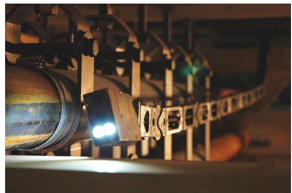
Figure 7: Inspection in a reactor of the Canadian nuclear power plant in Pickering (Ontario). © 2012 OC Robotics
