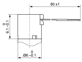
Figure 3 Dimensional Drawing [mm] – ENX 6 MAG
