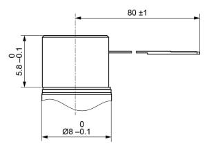
Figure 4 Dimensional Drawing [mm] – ENX 8 MAG
