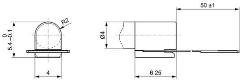
Figure 2 Dimensional Drawing [mm] – ENX 4 MAG
